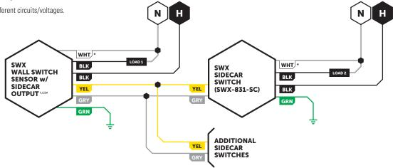
\* NEUTRAL CONNECTION IS OPTIONAL, CAP IF UNUSED 1 MODEL NUMBER SWK-102 INCLUDES UNIT SWK-101-SC AND SWK-831-SC 2 MODEL NUMBER SWK-121 INCLUDES UNIT SWK-111-SC AND SWK-831-SC 4 MODEL NUMBER SWK-122 INCLUDES UNIT SWK-131-SC AND SWK-831-SC
