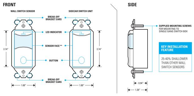
\*\* SENSOR FACE IS FIELD REMOVABLE IN ORDER TO CHANGE COLORS. CONTACT FACTORY FOR ADDITIONAL FACES
