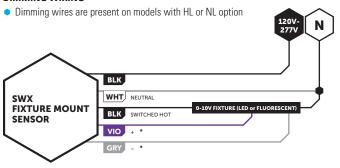
\* VIO/GRY DIMMING WIRES (0-10V) SHOULD BE TREATED AS CLASS 1
