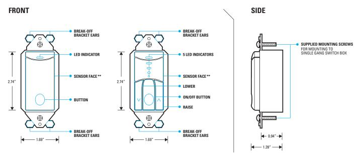
\*\* SENSOR FACE IS FIELD REMOVABLE IN ORDER TO CHANGE COLORS. CONTACT FACTORY FOR ADDITIONAL FACES
