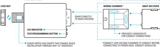
CONNECTING TO POWER PACK. CONDUIT SHOULD BE APPROPRIATELY SUPPORTED BY OTHER MEANS AND NOT USE THE LOW VOLTAGE CHAMBER FOR SUPPORT
