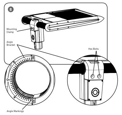
Numbers on angle bracket are shown for illustration purpose only. Actual bracket doesn't show numbers.
