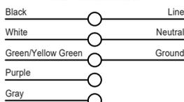
Note: Two dimming wires are in the driver box.
