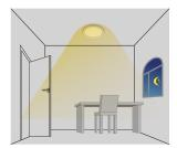
Light dims to standby level if no motion detected after holdtime.
