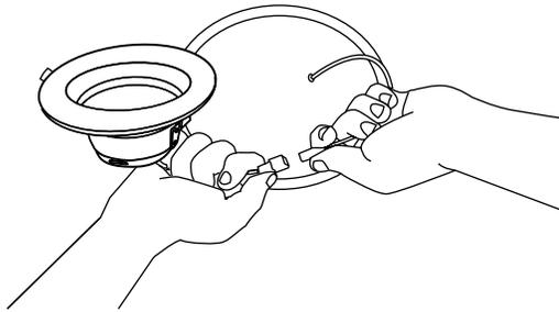
**4** If using an incandescent housing, screw the Edison base socket string into the socket. Mate the downlight connector into the Edison (or GU24) base connector.
