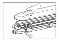
Unfasten the latches and remove the lens.
