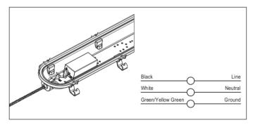
5. Connect the AC line to the black (line) and white (neutral) input wires of the LED driver . Connect the ground wire to the yellow green grounding wire, Connect the led strip wires to the driver .
