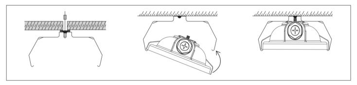
3. Mount the wraparound brackets on the ceiling or support rail using appropriate hardware. After brackets are secured in place, install one side of the housing in the bracket, then rotae up and snap the other side of the housing into bracket
