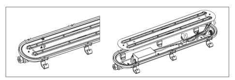
2. Loosen the screw nut, lift the LED board, then seperate the output wire of LED board from the output wire of driver.
