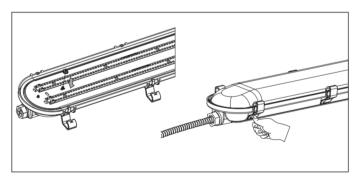
6. Twist the screw nut, put on the Lens Frame Assembly and tighten it.
