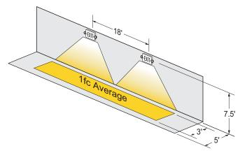
Using multiple units at a typical 7.5' mounting height with 80/50/20 reflectances on a 6' wide path of egress yields the following center-to-center spacing:
