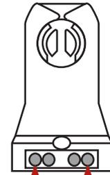
Connect wires directly to these terminals
