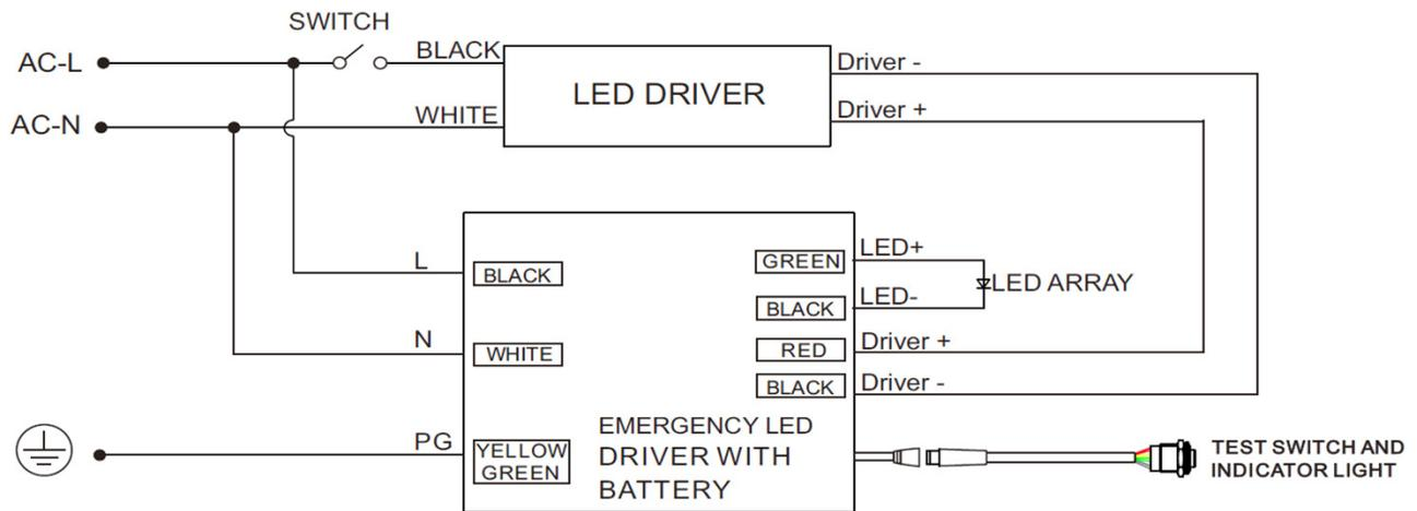
**AC LED driver output current cannot exceed 1A or 50W**
