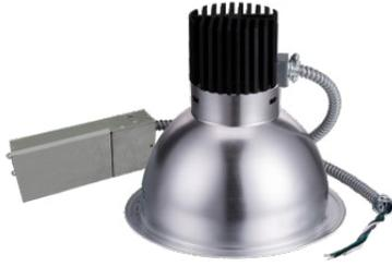
The **DC Commercial Downlight G2 Series** is a recessed downlight with Lumen adjustable features. This versatile downlight can be used in retrofit or new construction installations. The 0-10V dimming driver provides flicker-free dimming from 100% to 1%. Aluminum heat sink conducts heat away from the LED module for optimal performance and long life. Lumen packages range from 4,250 lumens to 6,800 lumens.
