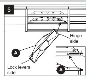
Hook the safety cables onto a hook or hole on the fixture housing as a secondary safety support.
