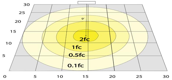
Simulation Based on 4000K Area 30'x 30' Mounting Height: 9'
