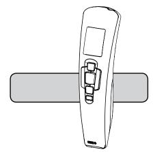
USB cable ( part number: LAH00206X0001A0 ) can be used to power the device in the absence of working batteries.
