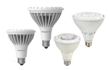
ULTRA LED HO PAR lamps deliver exceptionally high lumen output along with outstanding color uniformity and beam quality utilizing COB technology. Offered in a smooth heat sink, these lamps are available in a 15° spot, 25° narrow flood and 40° flood with the option of 120 or universal (120-277) voltage. The high CBCP performance makes these lamps a great replacement for high power halogen and HID lamps.
