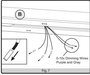
8. Connect the fixture wires to the supply wires -black to black, white to white, and green to
